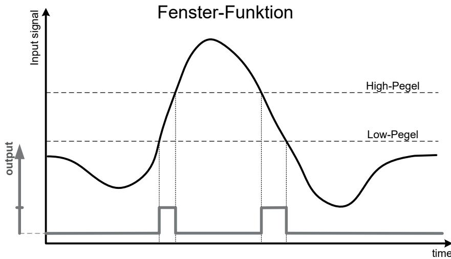
The fields “delay ON“ and “delay OFF“ doesn't have to be filled in necessarily. In the event of not entering a time the delay amounts 0 seconds each time. In case of entering a time (e.g. 5 sec), the monitored parameter has to be exceeded or to be fallen below the specified time before switching the warning channel.
