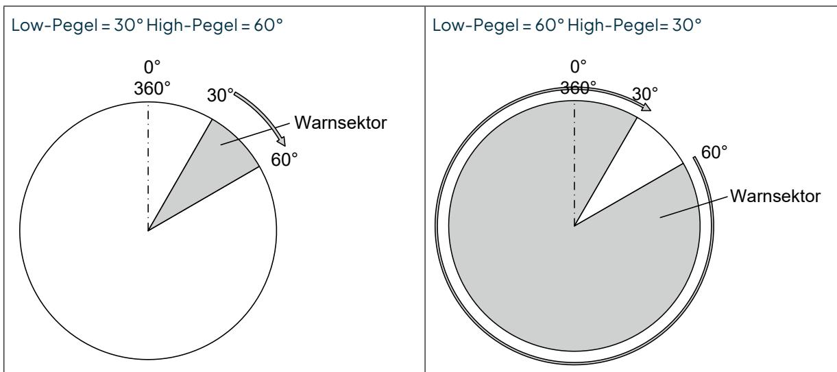
Alternatively, the in the example portrayed inverting can also be realized via the switch “inverted logic”.
